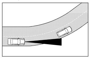
When following a vehicle and entering a curve, Adaptive Cruise Control could lose track of the vehicle in your lane and accelerate your vehicle. When this happens the Vehicle Ahead symbol will not appear.
